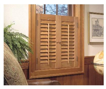
To determine the width of each shutter, take half the width of the window frame and subtract the width of the hanging strip and hinge used to atttach the shutter.
